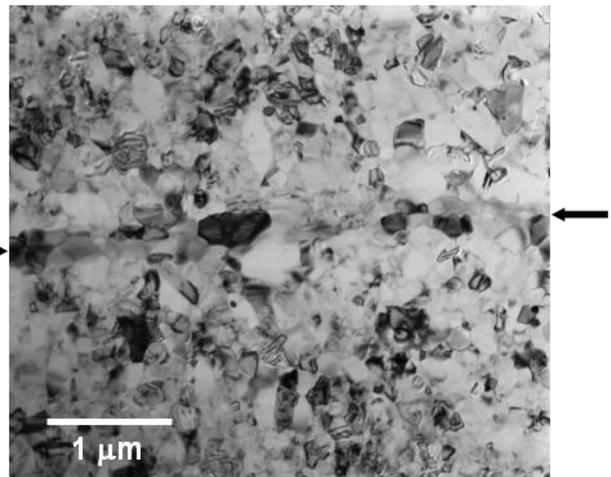
Fig. 3 – TEM micrographs of a TiAl joint processed at 900°C/ 50 MPa/ 1h using a Ti/Al multilayer thin film.
