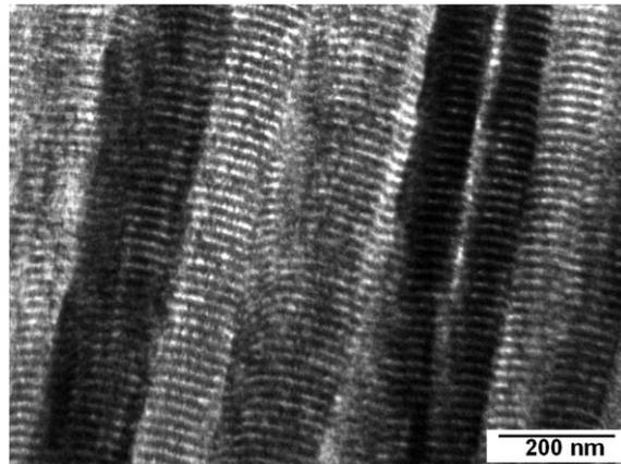
Fig. 2 – TEM micrograph of a sputtered Ti/Al multilayer thin film with 20 nm period.
