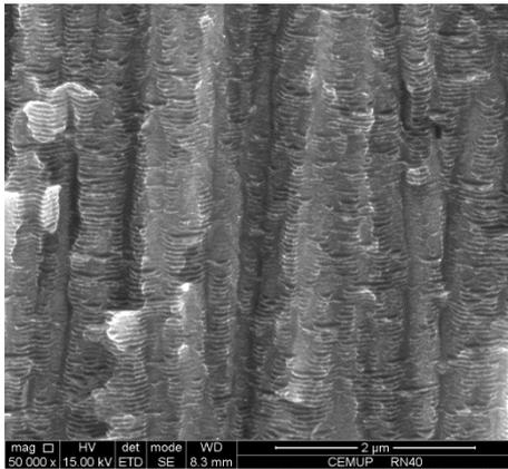
Fig. 1 – SEM micrograph of a Ni/Al nanofoil with 60 nm period.
