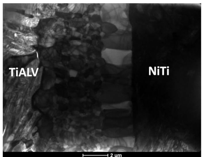
Fig. 5 – TEM micrograph of a NiTi/Ti-6Al-4V joint processed at 850°C/ 5 MPa/ 1h using a Ni/Ti multilayer thin film.
