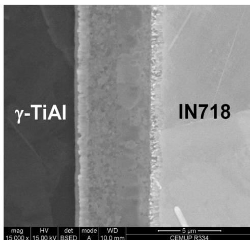
Fig. 4 – SEM micrograph of a TiAl/Inconel joint processed at 800°C/ 5 MPa/ 1h using a Ni/Al multilayer thin film.
